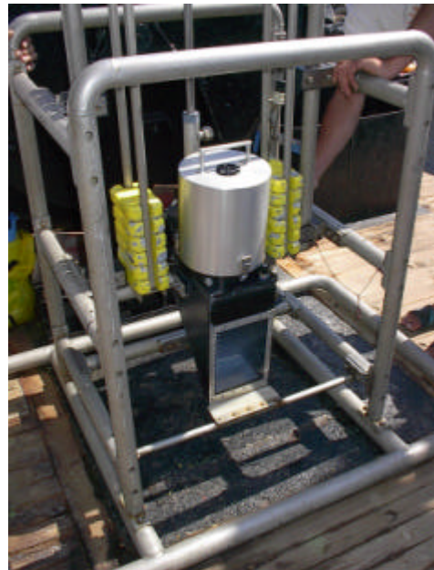
Figure 4. SPI Sediment Profile Imaging
