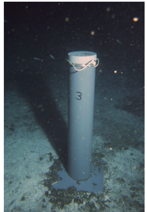
Figure 7. Sealed sediment trap on the sea-floor
